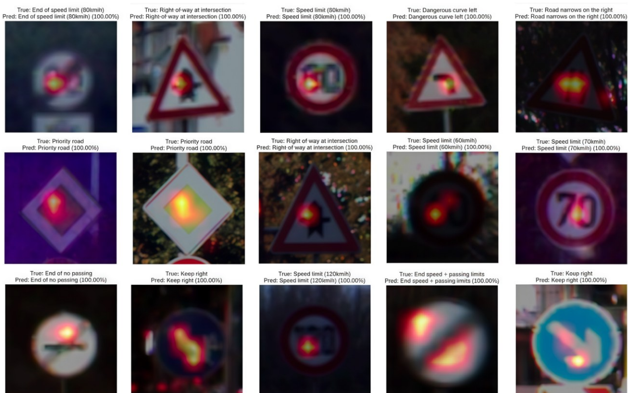
Figure 6. Grad-CAM interpretability analysis on the GTSRB dataset, highlighting the important regions of traffic sign images that contribute to the model's predictions.
